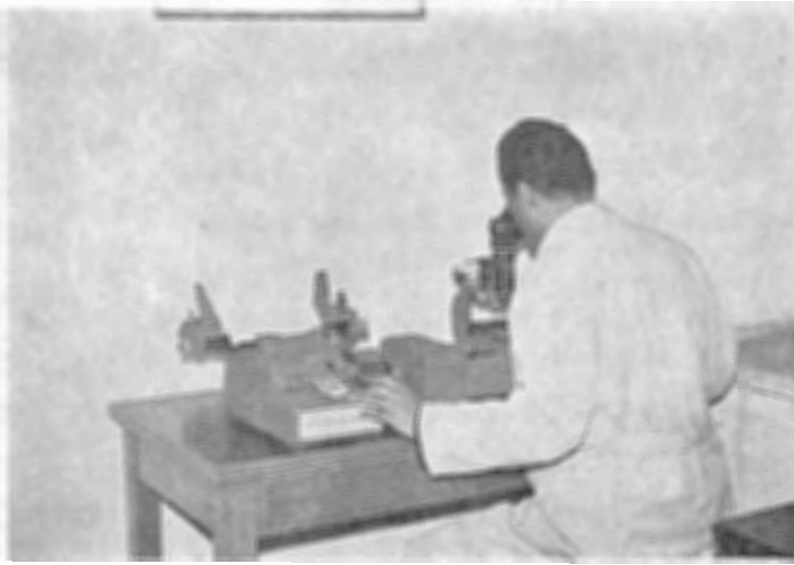
Figure 5. Annual ring counting machine in the forest management laboratory.
